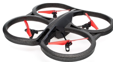
FIGURE 2.2: A quadrotor UAV, Parrot brand.
