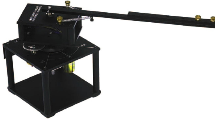
Figure B.1: The rotary flexible joint experimental setup made by Quanser.
